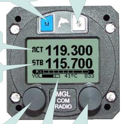
VOL/TEST knob. This provides adjustment of VOLUME. Pressing the knob inwards selects TEST and 'opens' the squelch. Holding this knob down enables further functions
