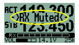
Radio volume is restored by holding the VOL/TEST knob down and rotating clockwise. Also, volume is automatically returned to normal by using the transmitter (pressing a PTT).
