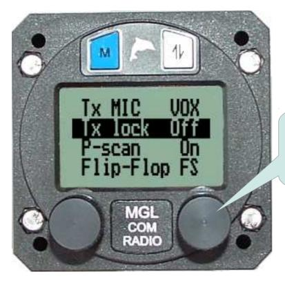
Rotate the knob to select the desired function and then press the knob inwards to adjust that function.
