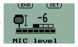
NB: For a single microphone, the level shown by the bargraph is for the Pilot microphone input ONLY. No level is shown for the passenger microphone. The adjustment affects all microphones equally.
