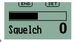
level between limits of -16 and +15. Adjust the squelch level so that static noise from the receiver is just 'squelched' out. Too high a level may result in weak transmissions not being received. Too low a level may result in noise breaking though. A setting is accepted by pressing the FREQUENCY knob.
