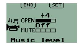
Open: This level applies if there is no audio from the intercom, the radio or the auxiliary inputs.
