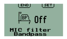
This can help reduce the effects of unwanted noise, in particular at low and high frequencies. This filter has a sharp cutoff for frequencies below 500 Hz and above 2.4KHz.
